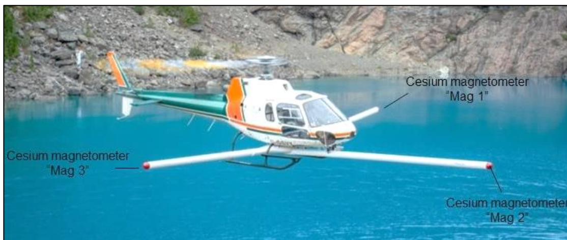
Figure 11: View of triple magnetic boom system.
