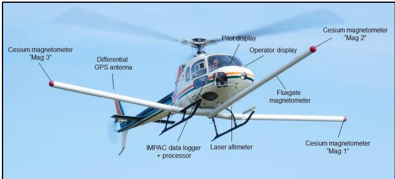
Figure 5 - Survey helicopter equipped with three magnetic sensors for gradient magnetic data acquisition.
