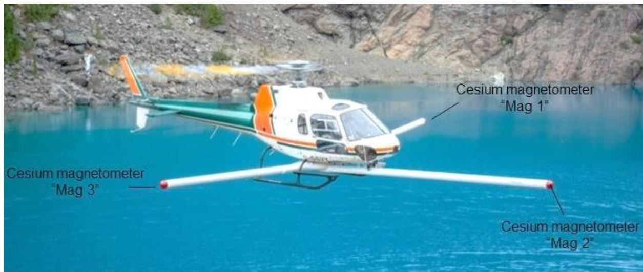
Figure 12 – View of triple magnetic boom system
