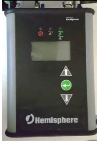
Figure 10 - Hemisphere R220 GPS receiver.
